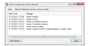
If the replication system is working correctly, the status will show **Ubisense Replication Service is running correctly**. You should also be able to see directories and files being stored in the dataset directory on the backup system, although this may take a little time to complete.
