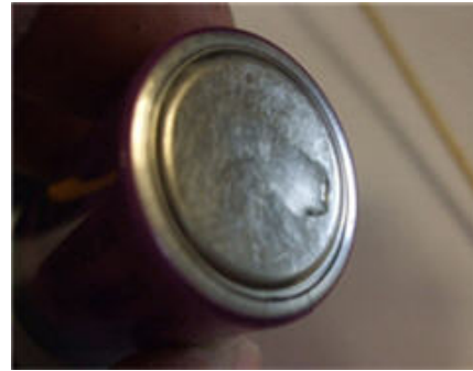
Too Much Treatment Oil Applied
