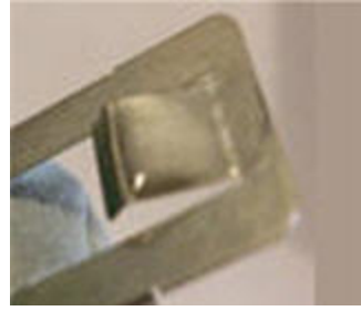
Too Much Treatment Oil Applied
