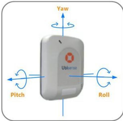
Figure 5-4: Yaw, Pitch, and Roll of a Sensor
