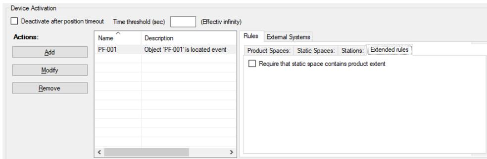
The Extended rules tab allows you to change how events are triggered from the default behavior described in [Rules in Combination](#).
