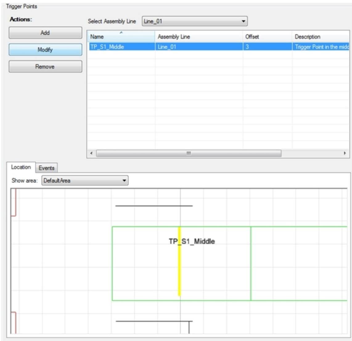
Figure: The Trigger Points Tab
