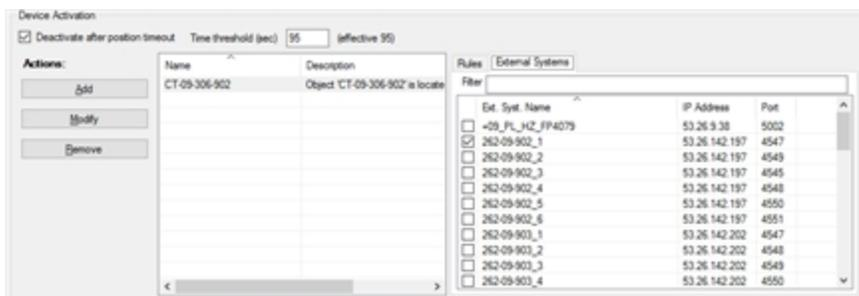
Use the External Systems tab to select an external system or systems to associate with the device instance. External systems are identified by their name, IP address and port. To associate a device with an external system, choose the check box to the left of the external system's name.
