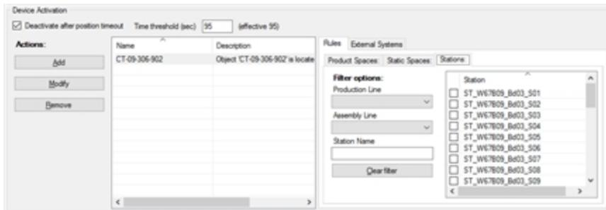
The **Stations** tab allows you to define whether a device is enabled for Station-driven-events.
