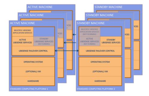
Multiple two-machine setups can be combined to cover a large system. In this case we have three active machines, each of which has a standby machine.
