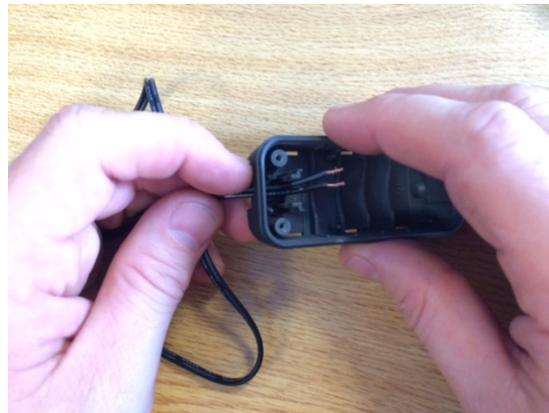
Passing the Wire through the Wire-entry Slot
