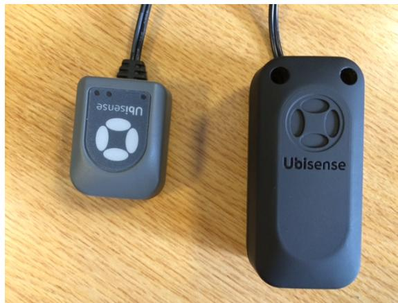
Assembled Head and Battery Unit
