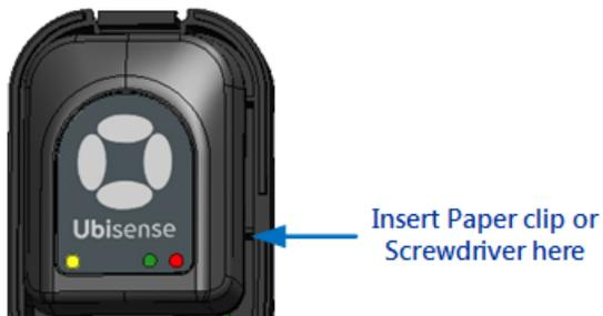
The yellow LED on the head unit slowly increases in brightness, indicating that the tag has been activated. After a few seconds the LED starts flashing to indicate that it is communicating with the DIMENSION4 Real-time Location System.
