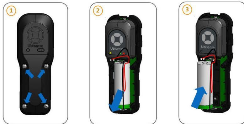
Replacing Battery of an Integrated Tool Tag
