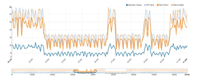
The line with focus is like the line chart, but designed for focusing in on specific ranges of the X axis. The chart is drawn with a range control underneath. Dragging on the range control selects the X range to show in the main chart.
