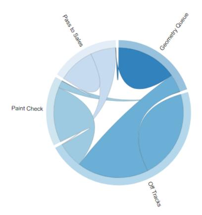
The chord flow chart also shows the number of objects making each possible state transition in the query data. As with the Sankey flow, the X column should identify a unique object, the Y column is a value than can be used to order the progress of the object, such as a time, and the Category column identifies the states, such as process steps.
