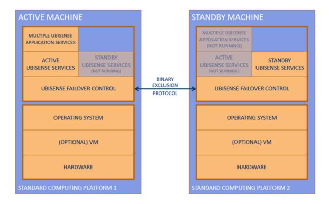
Figure: A two machine setup running a Ubisense system. At any one time, one machine is in the active state, and the other machine is in the standby state.
