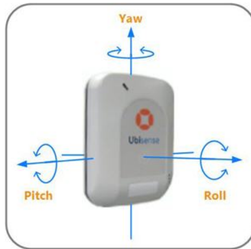
Figure 5-4: Yaw, Pitch, and Roll of a Sensor
