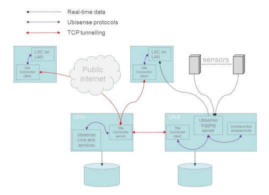
The important data paths to notice are the Ubisense protocols between the logging server and the analysis tools (run on the server) for historic analysis, and the real-time traffic between the logging server and the LSC on the LAN, for solver use and commissioning. Neither of these paths would touch the production server machine.
